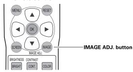
Brightness → Contrast → Color → Tint → Color temp. → Red → Green → Blue → Sharpness → Lamp control → Gamma → Progressive → Lens iris → Lamp iris → Auto black stretch → Contrast enhancement → Transient improvement → Gain R/G/B → Offset R/G/B → Gamma R/G/B → Brightness → ....
