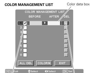
Clear the check mark if you do not want to apply this adjusted color data to the projected image. Select the DEL box if you want to delete the adjusted data. A confirmation box appears.
