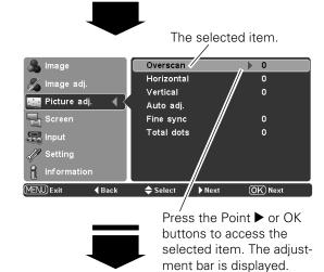
Use the Point ◀▶ buttons to adjust the the setting values and press the OK button to return to the submenu.
