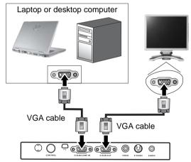
The D-Sub output only works when an appropriate D-Sub input is made to the projector.
