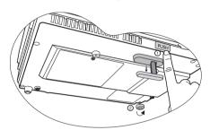
To retract the foot, hold up the projector while pressing the front adjuster button, then slowly lower the projector. Screw the rear adjuster foot in a reverse direction.
