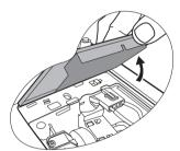
4. Disconnect the lamp connector from the projector.
