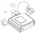
Do not operate lamps beyond the rated lamp life. Excessive operation of lamps beyond the rated life could cause them to break on rare occasions.
