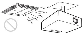
Installing the projector in such a location may cause a malfunction of the unit due to moisture condensation or a rise in temperature.
