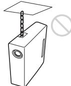
Use the Security bar at the rear of the projector for a purpose of preventing theft, by attaching a commercially available theft prevention cable for example. If you lift the projector by holding the Security bar, or hang the projector by using this bar, it may cause the projector to fall or be damaged.
