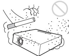
Avoid installing the unit in a very dusty or extremely smoky environment. Otherwise, the air filter will become obstructed, and this may cause a malfunction of the unit or damage it. Dust preventing the air passing through the filter may cause a rise in the internal temperature of the unit. Clean the air filter whenever you replace the lamp.
